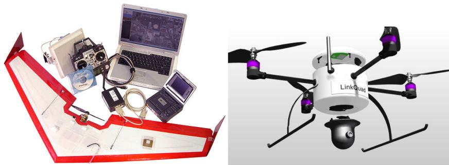
**Fig. 1.1** The depiction of the *Procerus* UAV kit and the *LinkQuad* quad-rotor VTOL employed in the on-going research projects of the *Agent Technology Center*.
