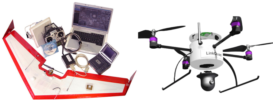
Figure 4. AgentFly UAV hardware platforms. Left, Procerus fixed-wing aircraft with the development toolkit; Right, LinkQuad vertical take-off and landing quad-rotor aircraft.
