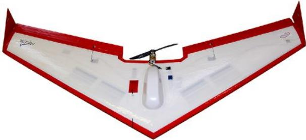
Fig. 4: Unicorn fixed-wing UAV from Lockheed Martin
