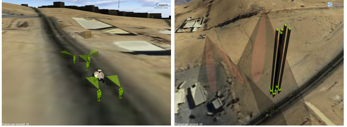
Figure 4.11.: The ground forces (green) supported by the robotic team (2 Vidar VTOL MUASs – orange, 2 Skeldar VTOL UASs – red, 1 MDARS UGV – brown) in the simulated urban environment.
