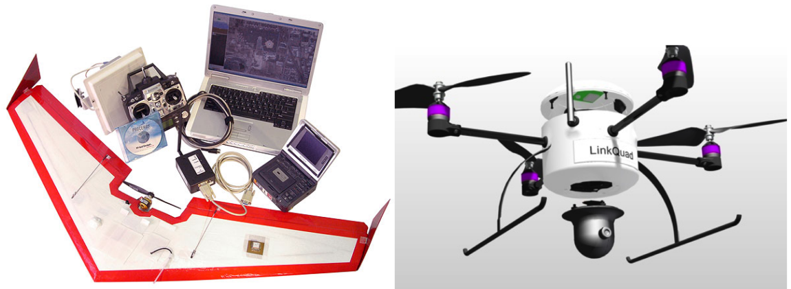
Figure 1.1.: The depiction of the Procerus UAV kit and the LinkQuad quad-rotor VTOL employed in the on-going research projects of the Agent Technology Center .
